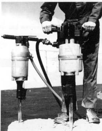
The 1980's .... The "Big" TEX50 (right) with vibration damped handles.
